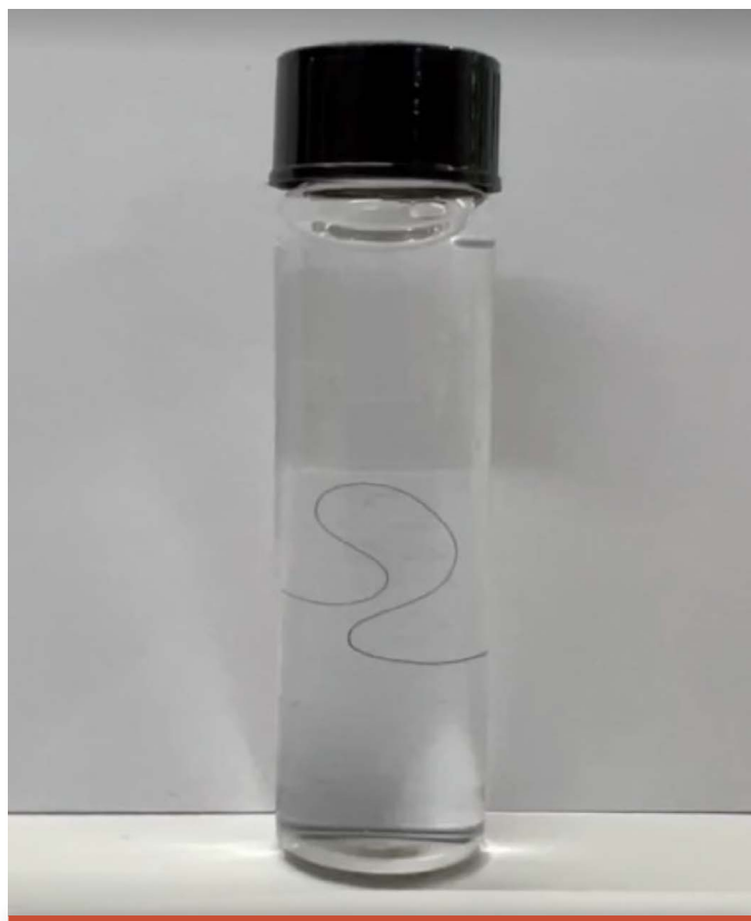
Image: A hydrogel microelectrode. Credit: Rao Lab .
