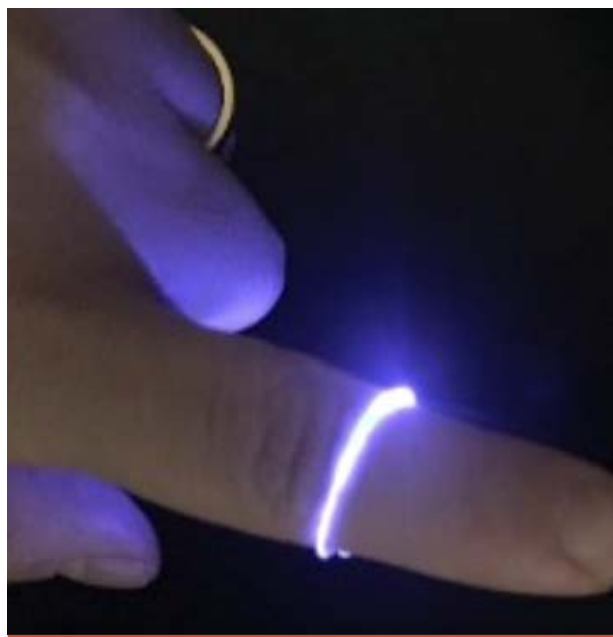
Image: Soft multifunctional neuro probes wrapped around a finger. Credit: Rao Lab .
